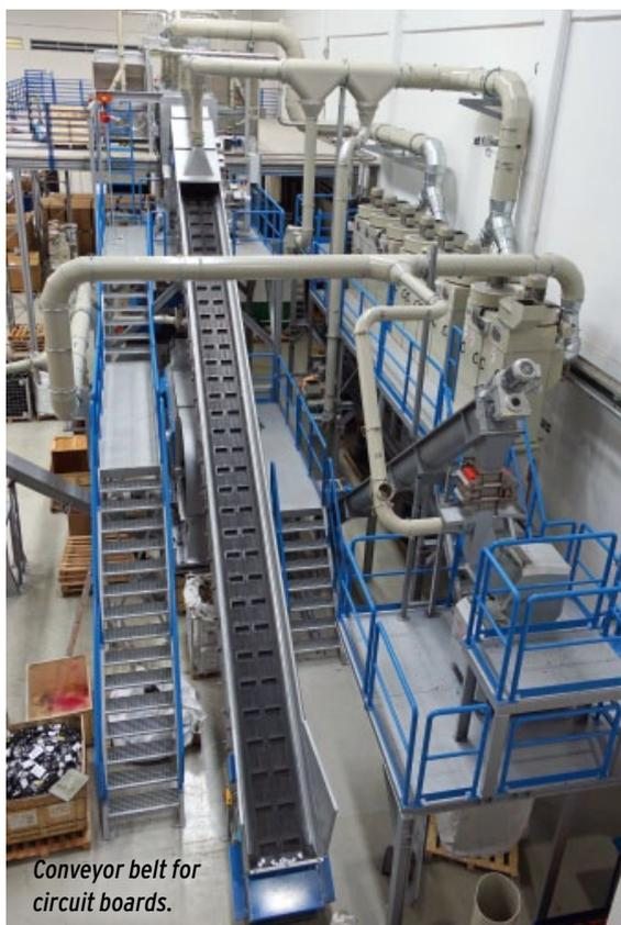
Conveyor belt for circuit boards.
