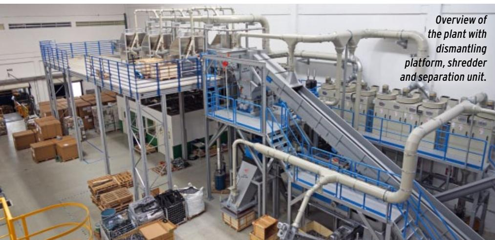
*Overview of the plant with dismantling platform, shredder and separation unit.*
