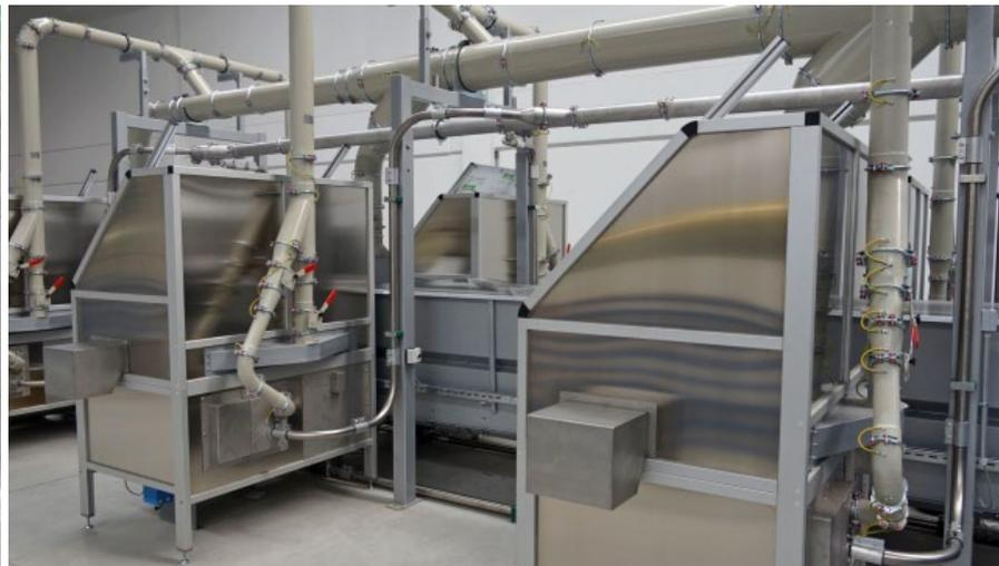
Layout of the dismantling cabin at the conveyor belt to the cartridge shredder.
